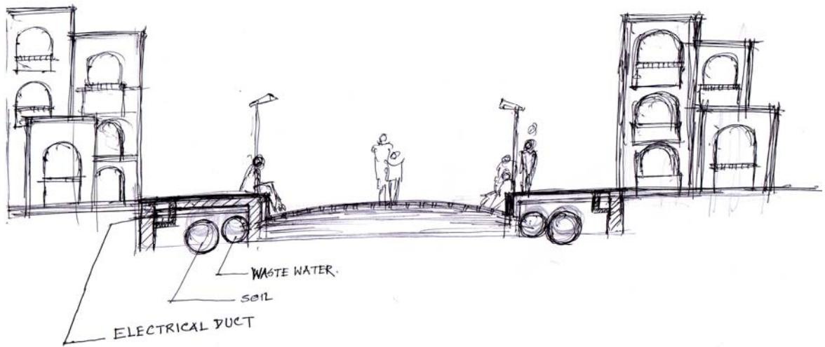
X- section of the proposed walkway showing the underground utilities provision
