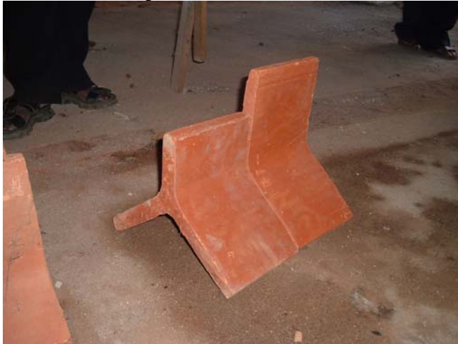
Specially manufactured ridge tiles based on original design
