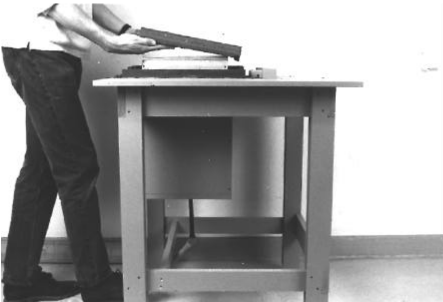
Use the foot pedal to lift the tile together with the base sheet.
