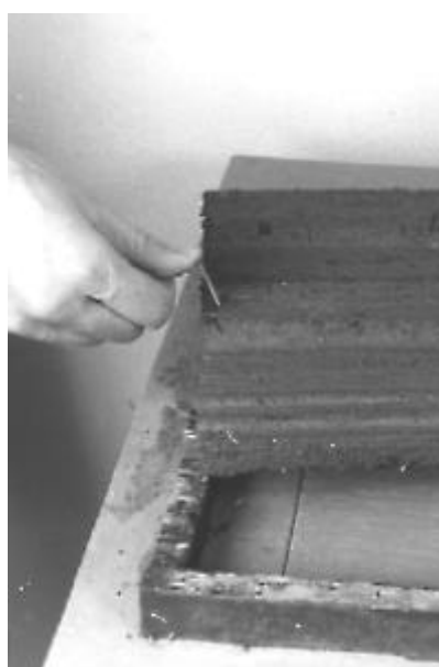
Before taking the tile to the curing room, cut off the corner and, if needed, use a nail to make a hole for fastening the finished tile to the roof batten.
