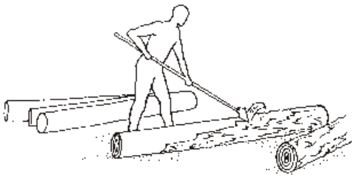
Fig. 6 Debarking the tree trunks before they are air dried.
