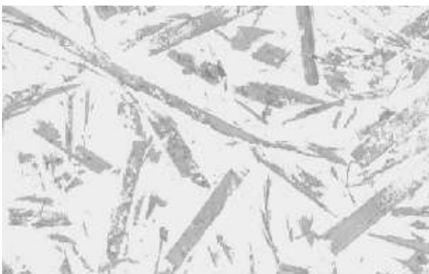
Fig. 5 Slab coated with gypsum plaster, resulting in a smooth surface that retains the texture of the slab (Climatex, Brazil).
