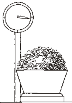
Fig. 11 Woodwool is weighed manually before soaking.
