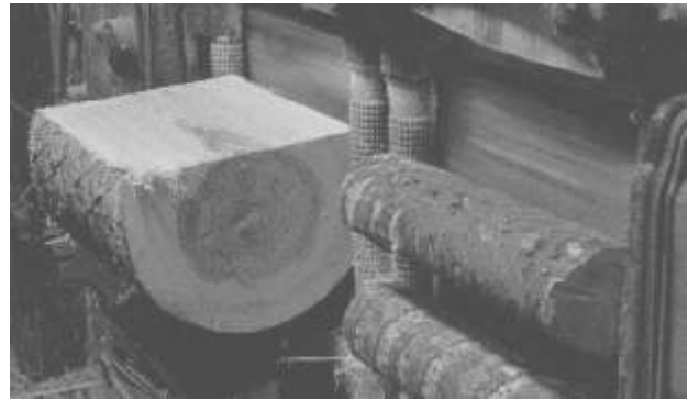
Fig. 1 Making woodwool in a vertical wood shredding machine (Tepro, Sweden). Shredders sold today are horizontal. See Figs 9 and 10.
