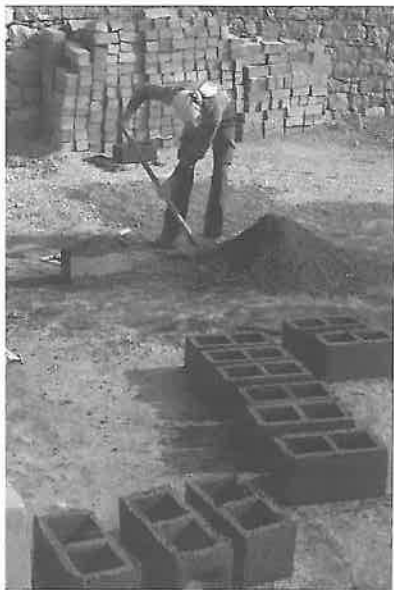
Making hollow concrete blocks
