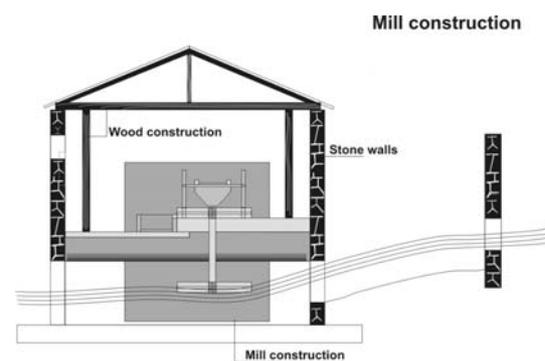
Fig 5. Technological scheme of Stolac mill
