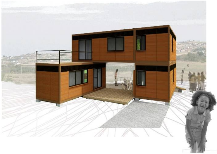
Fig. 7 - Enlarging: The system allows vertical and horizontal expansions. The modules can be done by the users as it is an open system. Materials can be easily acquired at reasonable cost in the open market (plywood, wood, nails, etc)
