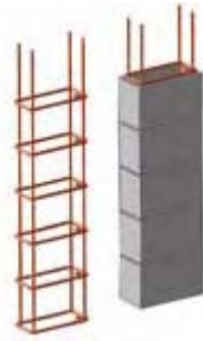
Picture 7 - Column HCB with reinforcement
